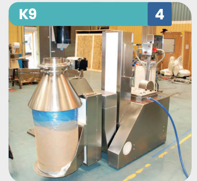
Electrically propelled mobile truck for gripping lifting and inverting drums and IBC's, Bins and Totes up to 250kg
