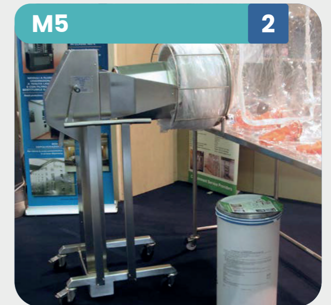
Fixed mast manually propelled mobile truck with manually actuated drum raise, lower and forward pour
